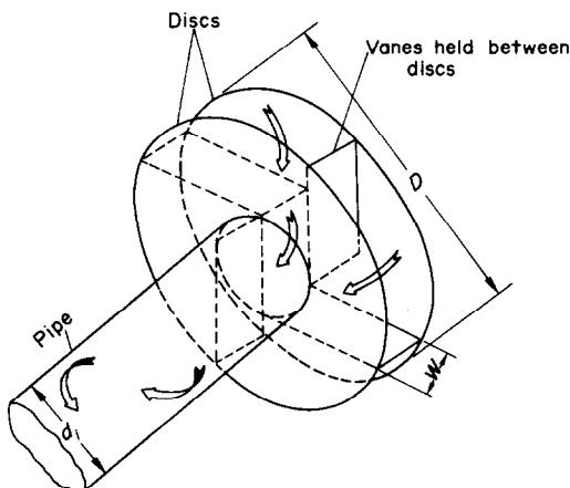
FIG. 1. Tangential vane swirl generator.
