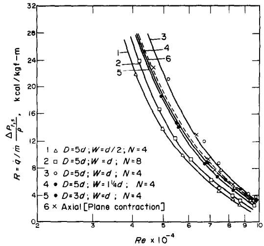
FIG. 6. Ratio of heat-transfer rate to pumping power,  $R$ , for different swirl generators.
