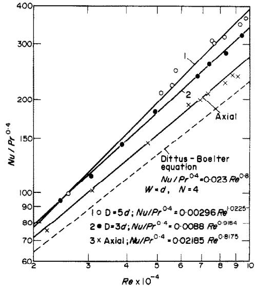
FIG. 4. Effect of swirl generator diameter on the average Nusselt number.
