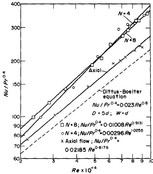
FIG. 5. Effect of number of vanes of the swirl generator on the average Nusselt number.
